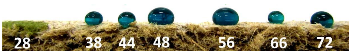
Figure 8 : Tests encres – échantillon ET-20%MMB-HMDSO.
